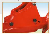
Different type of soil and moisture content, all have different demands for working width. For this easy and quick adjustment is given. It can be adjusted for 10", 12" and 14".
