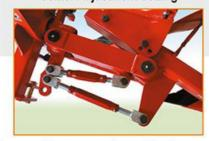
Center adjustment setting makes it easy to adjust front furrow width and tractor pull line independently of each other.
